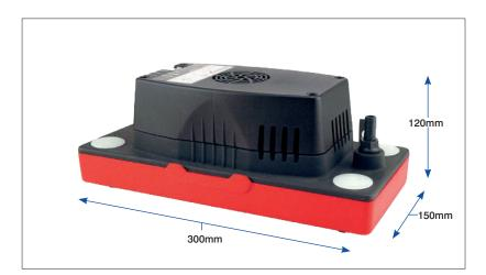
The DiversiTech RedBox 1 Litre Tank Pump is a condensate tank pump with a flow rate of 280 LPH and a lift of 5.1 metres. This pump has metal mounting tabs which allows the tank to be screwed to the wall. The universal power lead makes the pump easy to install, service and retrofit.
