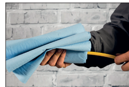
STEP 4 These benders are reusable if wiped clean between installations.
