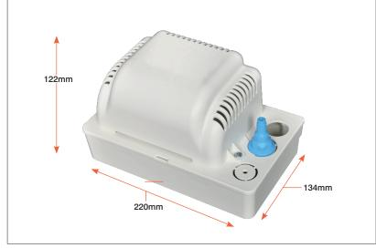
When space and lift are a challange, our shallow tank pump enables installation in compact areas such as below kitchen units. The 6 metre discharge lift helps with the flexibility of the installation. Suitable for both floor and wall mounting and comes with a quick release check valve. Suitable for boilers up to 100kW.
