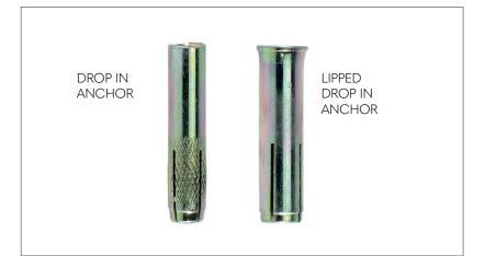
Deformation controlled zinc plated and yellow passivated Drop In anchor is an internally threaded socket suitable for applications in non-cracked concrete. Full expansion can be guaranteed by using the correct shouldered setting punch. Internal thread suitable for bolts or threaded studs of any length. Lipped Drop In anchors can be accurately set independent of the hole depth and can be used in concrete.
