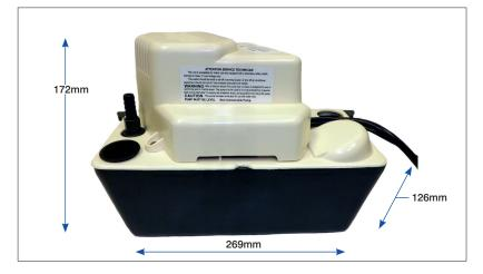
The economy option in 2 litre tank pumps, this low-cost centrifugal pump is designed to remove condensate water from air conditioners, refrigeration equipment and de-humidifiers. Fully automatic with a 1/4" & 3/8" non-return valve, this economy condensate pump delivers a maximum flow of 275 litres per hour with a maximum head of 3.8 metres.
