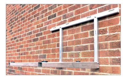
These flat-packed, self-assembly stainless steel brackets provide a professional finish to the installation of wall-mouted outdoor condensing units and air source heat pumps. The Type 2 brackets have a crossbar allowing the uprights to be spaced exactly as required, and include wall spacers to help level the unit on uneven walls.
