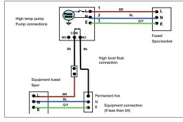
Boiler connection to the high-level safety switch
