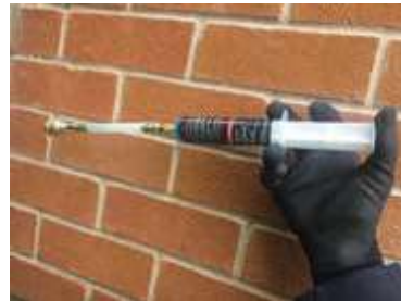
4. Push down syringe plunger to remove air from hose and remove bleed fitting.
